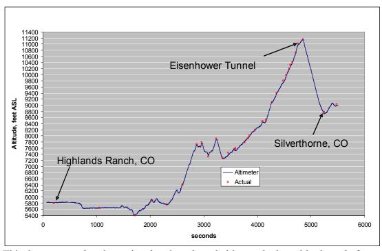
This data was used to determine that the selected altimeter had an altitude scale factor that was low by 0.68%.
