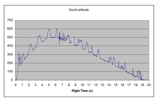
The rounded spikes in the data occurred when the pressure sensor was facing the sun. From this data it can be inferred that this rocket rolled 6 revolutions on the way to apogee.
